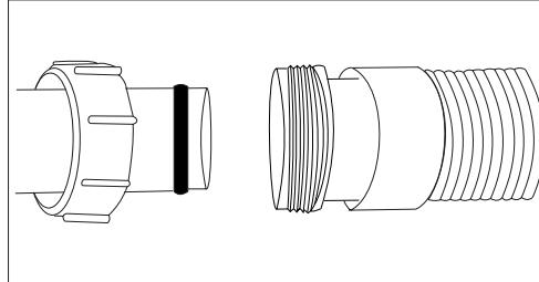
6/ Reassemble the nut and seals from the Flexi Pipe onto the pipework.
