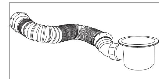
4/ Extend and shape the Flexi Pipe as required ensuring a drainage gradient of not less than 1 in 40 without sagging.
