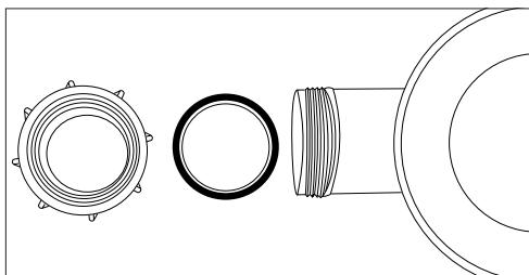
1/ Using a suitable waste unit having a 40mm compression fit connection, disassemble the nut and seals from the unit.
