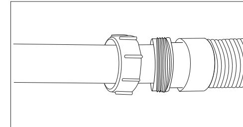
7/ Ensure the pipework is fully inserted into the Flexi Pipe and then tighten all connections.
