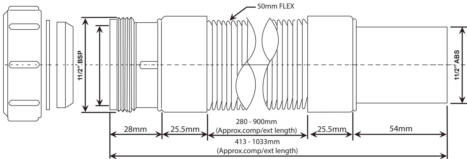
Your Flexi Pipe is an essential part of almost any shower tray plumbing system in tricky installations where rigid piping would be difficult to fit, adjustable from as little as 413mm out to 1033mm offering versatility in tight or awkward spaces.
