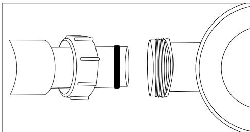
2/ Reassemble the nut and seals from the unit onto the unthreaded open end of the Flexi Pipe.
