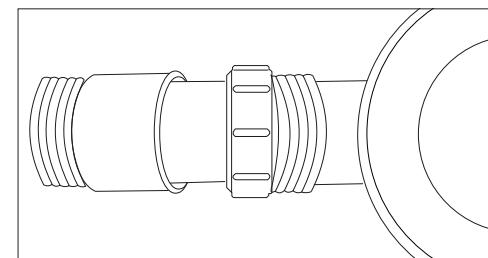
3/ Attach the Flexi Pipe to the waste unit ensuring that the end is fully inserted into the unit and then ensure all connections are tight.
